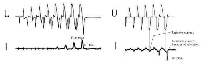
All measurings are made on primary coil at 230V
