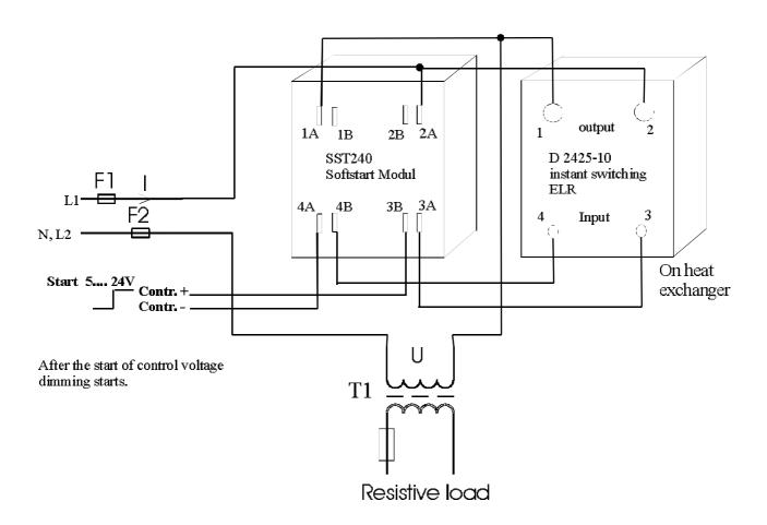
1kVA EI Transfo, 1,3 tesla Ind. with progressive sym. Dimming switch on Current peaks when Transfo is not full loaded 1kVA Toroid softstarted with progressive sym. dimming Loaded with nominal load. Transformer is going into saturation.
